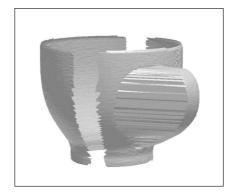
Example of starting from the front at an angle (two scanning surfaces)
